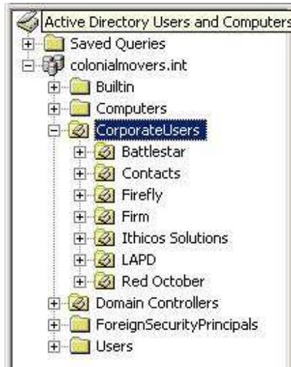
Figure 7: OU structure for an Active Directory
